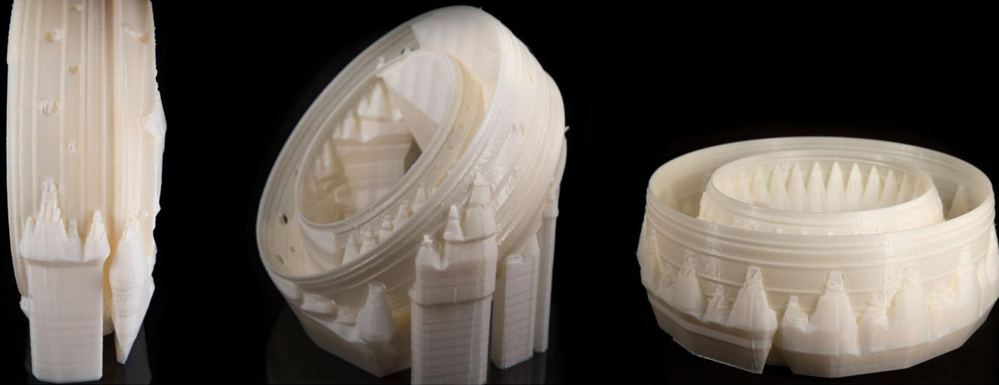
Combustion liner prototype build at three different orientations.
