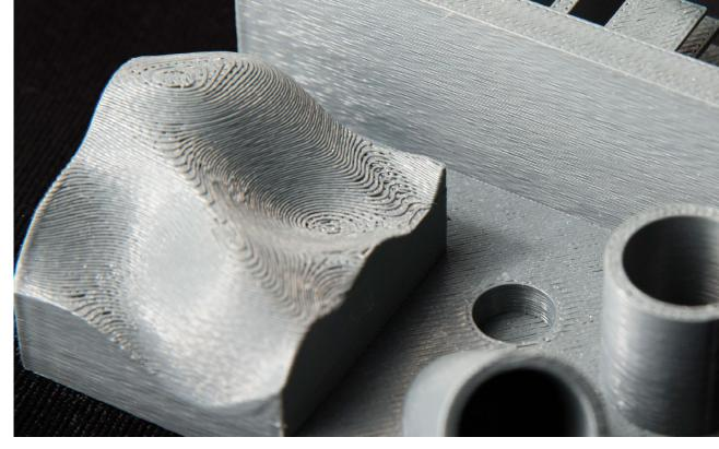
Layer resolution is the thickness of each slice laid out during the build of a 3D printed prototype.
