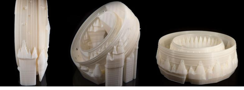
Combustion liner prototype build at three different orientations.
