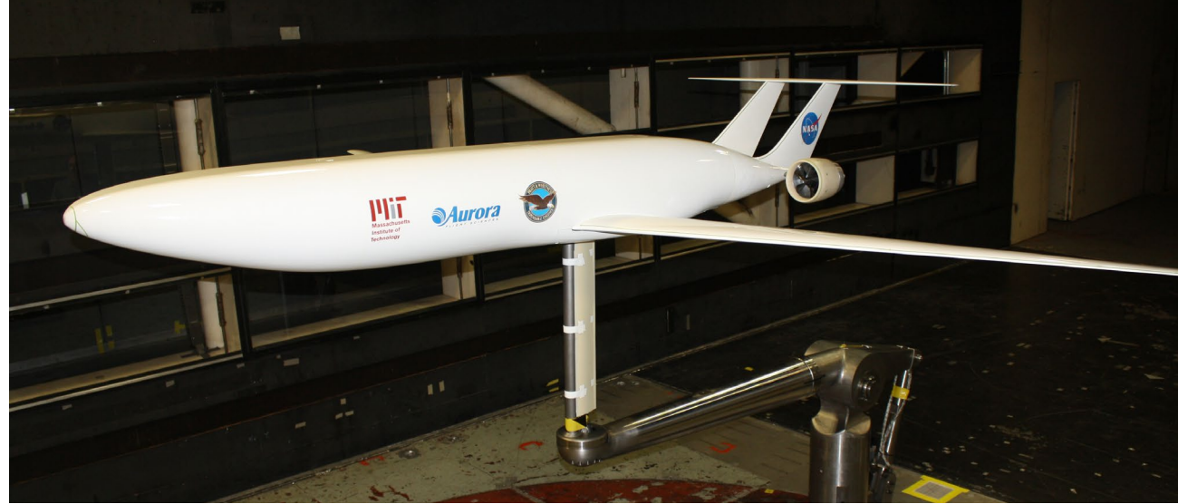
NASA N+3 wind tunnel model.
