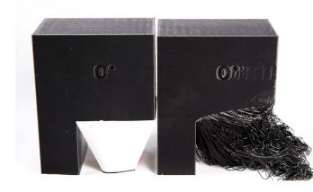
O degree angles require support material or significant failures will occur.
