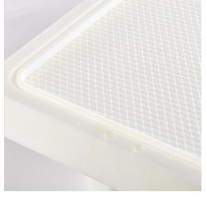
Sparse fill in FDM parts can lightweight parts and reduce required material.
