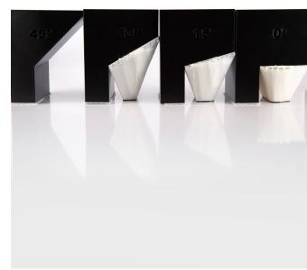
Various angles with support material. 45 degree angles do not require support material.
